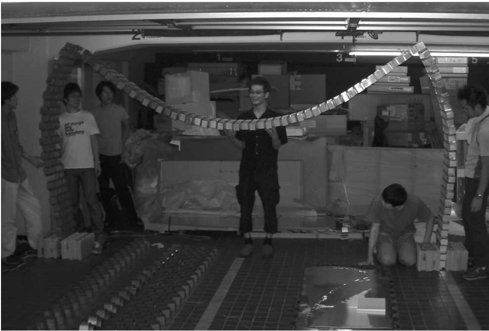
Figure 12. Deflection of honeycomb was tested through full-scale mock-ups (© Toyo Ito & Associates).
